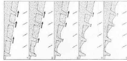
Evolution of Planform on Littoral Drift Coast (Source: Stephens, Roy and Jones, 1981)
